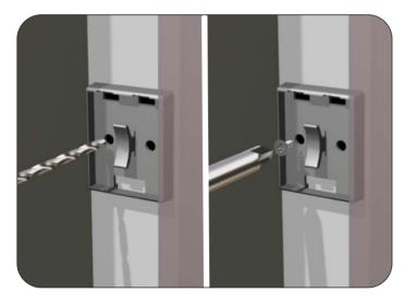
6. When the back of the cord lock is fitted, use two screws to secure the cord lock.
